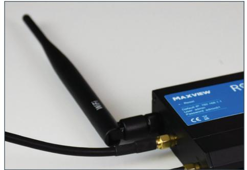
4. Attach the Wi-Fi antenna to the top connector. This is marked 'Wi-Fi'. This should be positioned so it is vertical.
