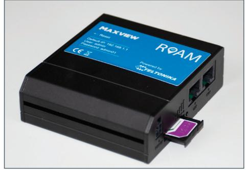
2. Use the Needle Pin to remove the SIM card holder. Place your SIM card of choice in the holder and slide back into the router. See page 4 for more information on SIM card preferences.
