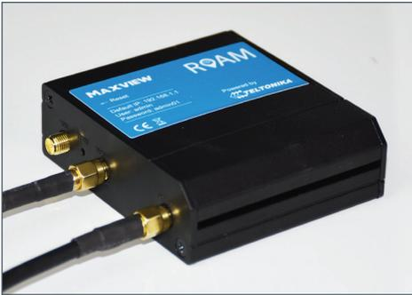
3. Attach the antenna coaxial cables to the bottom 2 connectors. These are marked 'mobile'. Note the order of the cables does not matter.
