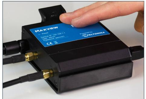
6. Place the router into the mounting bracket. The router can be removed from the bracket at any time to change the SIM card as required.
