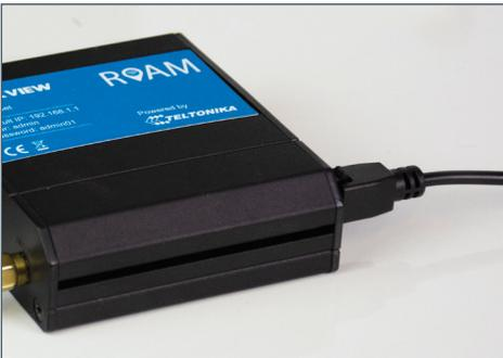
5. Connect the 12V power lead or the 230V PSU and route the lead to your power source.
